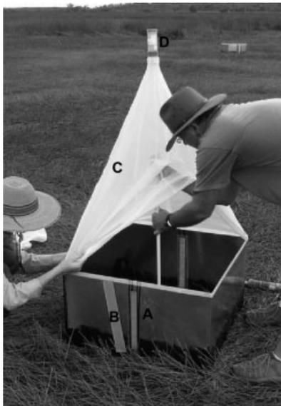
**Figure 2.** Emergence trap design: mesh-covered holes allow tidal flooding without larval movement (A); yellow magnets applied over holes prevent unwanted larvicide from entering the trap (B); mesh emergence tent prevents unwanted species oviposition inside the trap (C) and also catches emerging adults (D).
