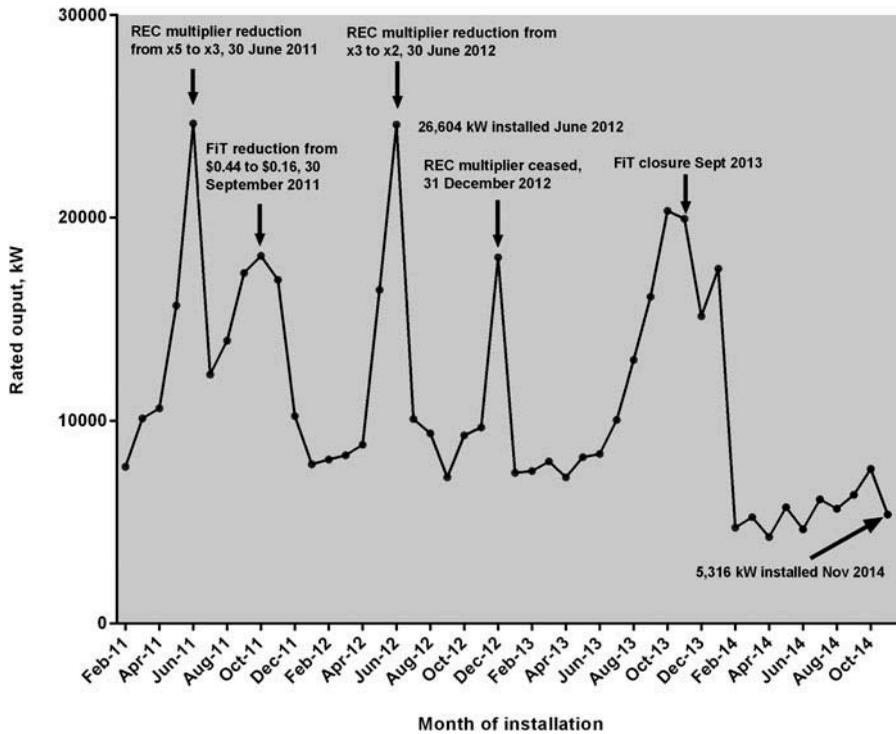
Figure 6. Monthly solar photovoltaic installation in South Australia ( $\text{kW month}^{-1}$ ) from February 2011 to November 2014 showing reduction and withdrawal Renewable Energy Certificate (REC) multipliers and Feed in Tariff (FiT). Sources: Clean Energy Regulator (2012), Clean Energy Regulator (2014c).
